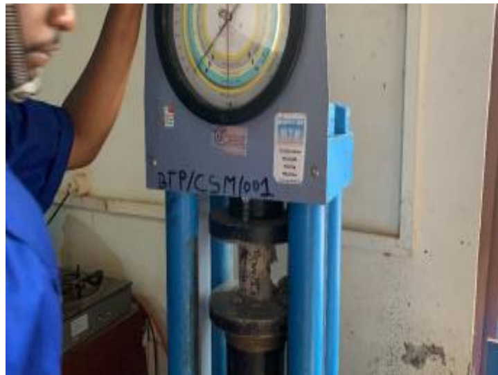
Figure 2: Compression testing machine in supporting transmission tower operation of testing concrete cores.
