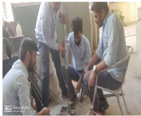
Figure 6. Mix placed in mould compacted and bitumen
