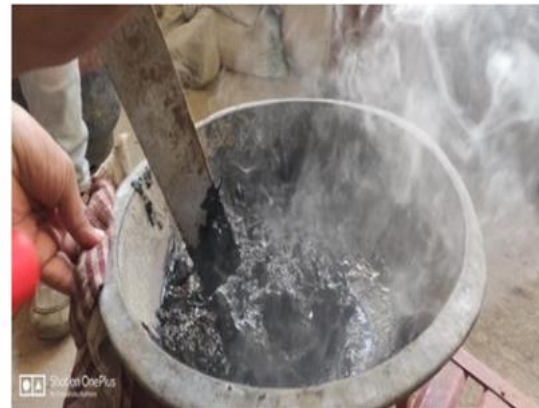
Figure 4. Molten plastic slurry
