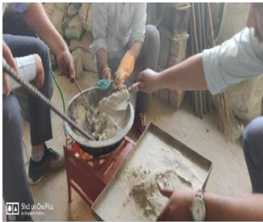
Figure 5. Fly ash being mixed in melted plastic
